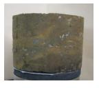
Note: A B-value of 0.96 was achieved for the undisturbed specimen. Permeation measurements were made with a mercury U-tube. The effective confining pressure was 5 psi per test request.
