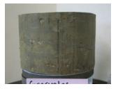
Note: A B-value of 0.95 was achieved for the undisturbed specimen. Permeation measurements were made with a mercury U-tube. The effective confining pressure was 5 psi per test request.
